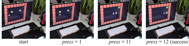
Fig. 1: The hand combines untethered locomotion with self-supported interaction. Top: locomotion demonstrated on 14 surfaces: (a) rubber mat, (b) carpet, (c) hardwood, (d) tile, (e) diamond plate, (f) metal grating, (g) hard court, (h) asphalt, (i) dry concrete, (j) cut stone, (k) weathered stone, (l) artificial turf, (m) grass, and (n) gravel. Bottom: self-supported manipulation: (o) 12 keyboard presses completing a Sokoban level; (p) object pushing from approach through delivery.
